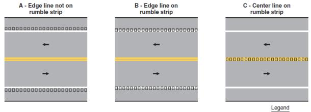
Figure 3J-1. Examples of Longitudinal Rumble Strip Markings
