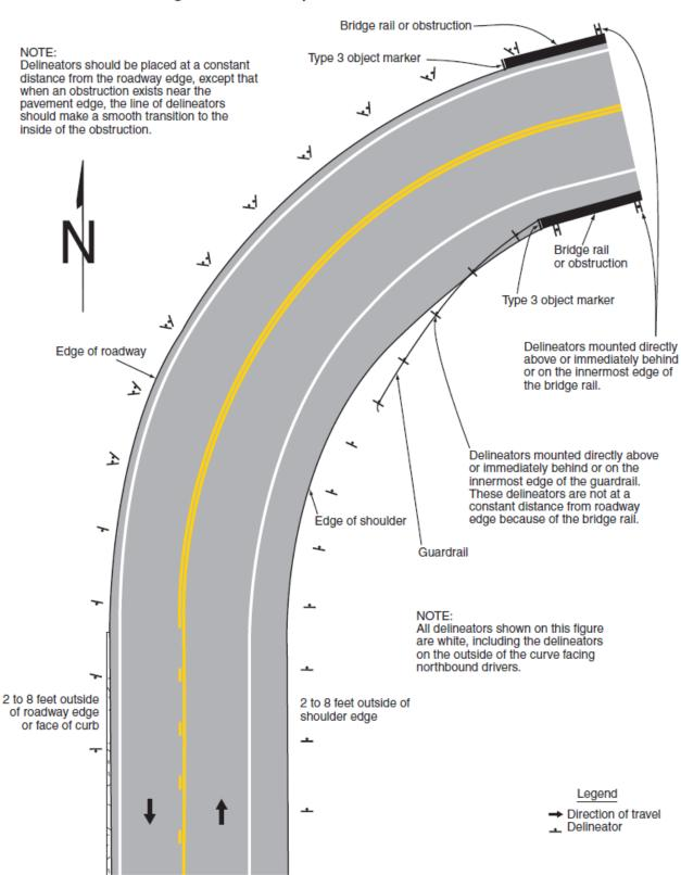
Figure 3F-1. Examples of Delineator Placement
