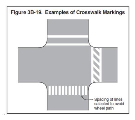
At locations controlled by traffic control signals or signs, crosswalk lines should be installed where engineering judgment indicates there is a need. An engineering study considering the following factors should be performed before a marked crosswalk is installed at a location away from a traffic control signal or sign. These pavement markings should never be used indiscriminately.
