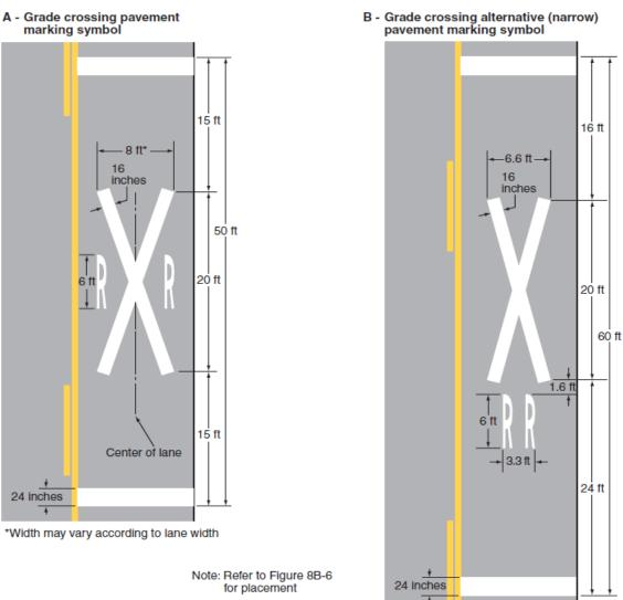
Figure 8B-7. Grade Crossing Pavement Markings
