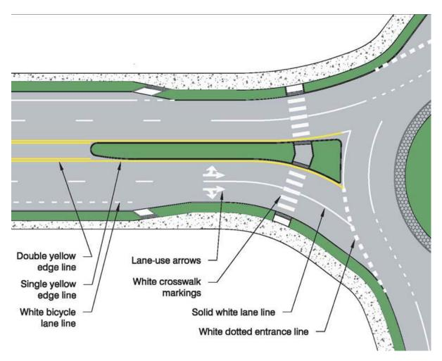
**Yellow edge lines** should be used along splitter islands on the left edge of entries and exits, as well as the left edge of right-turn bypass roadways.
